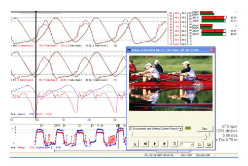
Peak forces are matched well, even though the two scullers are slightly dissimilar in force curves, with the stroke being somewhat simultaneous and the bow being sequential. Leg kinematics are identical.
