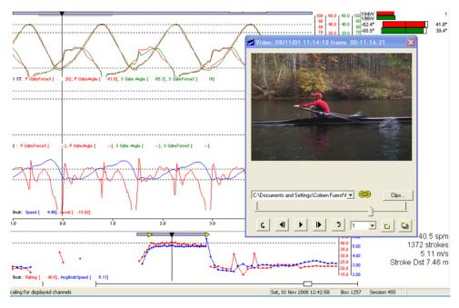
Shown directly above are 2 screen grabs taken from a force measurement system data logger printout. One is of a double and the other of a single with video syncing. Referring to either: The very top graph(s) shows a large red/green
