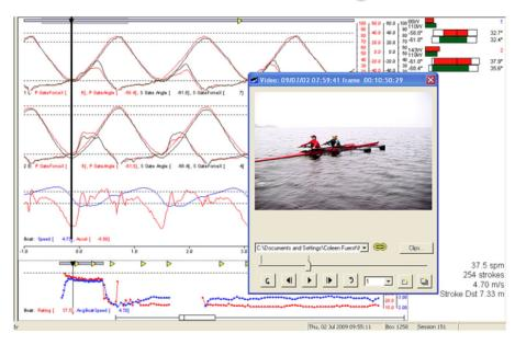
The next graph shows that acceleration has just started, along with force just starting to be applied, however the stroke length bar chart shows a large slip (slow catch) from the bow position relative to the stroke and the video reveals a corresponding not fully buried blade at bow.
