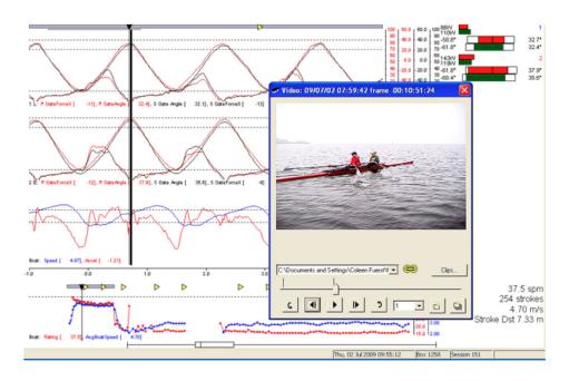
The first thing to notice about the heavyweight men's double is how quick their catch is, with the maximum gate angle and the true catch being virtually indistinguishable on the graph or in the video. Only the hands raise with no other body movement. The stroke length bar chart confirms that with very little or no white area showing at full extension of -70°.
